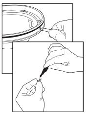
NOTE: If you are installing an outdoor model, plug the two-pin heater connection in the lower dome into the mating connector in the back box.
